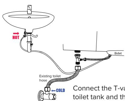
Connect the T-valve under the toilet tank and the two hoses. Connect the thinner hose to the hot water supply under the sink. Tighten.
