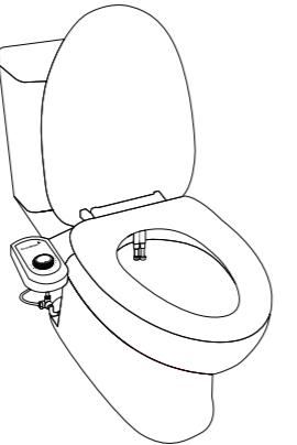
Turn on the water supply. Check to see if it is installed properly and works properly.
