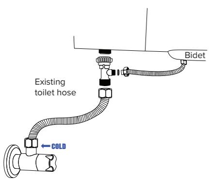
Connect the T-valve under the toilet tank and the two hoses. Tighten.
