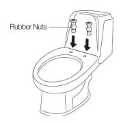
Place the bolt cases onto the baseplate then place the mounting bolts through the bolt cases. Screw bolts into rubber nuts with a screwdriver and tighten.
