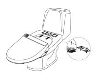
Connect the plastic tube from the side of T-Valve to the side of the SmartBidet and tighten. Turn on the water supply and watch for any leaks.
