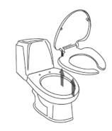
Connect T-Valve directly under toilet tank. NOTE: DO NOT CONNECT T-VALVE TO WATER SUPPLY VALVE AS INDICATED ON PAGES 15, 16 IN THE MANUAL.
