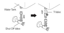
◆ Connect the metal hose to the T-valve and water supply valve. Tighten. NOTE: The end of the hose's diameter is 3/8". Please check if your water supply valve's diameter is the same. All bathrooms water supply valves are not the same. If it is not, please purchase an adaptor that fits at your local hardware store.
